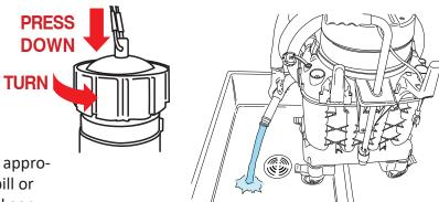
Once cap is removed, lower Dump Hose into appropriate sink/drain. To prevent an accidental spill or overflow from the Dump Hose, be careful to keep hose end upright until it is over sink/drain.
