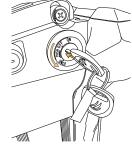
Push key IN and rotate counter clockwise to Unlock.
