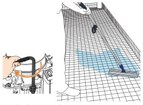
Turn Spigot clockwise to the OFF position. Use Spreader Tool in back-and-forth motion to cover floor with cleaning solution. \*Agitate Spreader Tool over troubled or extra soiled areas to get a deeper clean\*
