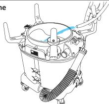
Fill the tank with water and recommended amount of **Kaivac approved Chemicals**. Follow the proper dilution instructions on bottles or dispenser. For accuracy and convenience, use Kaivac proportioned chemical packets.
